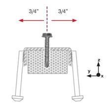
Figure 7 — Allowed screws position on HAC-TU along the perpendicular (y) axis
