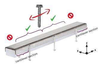
Figure 6 — Allowed screws position on HAC-TU along the longitudinal x) axis
