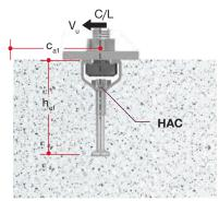
Figure 4a — Edge distance ( $C_{a1}$ ) of a cast-in anchor channel such as HAC (figure for illustration purposes only)
