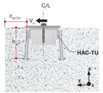
Figure 4b - Edge distance (Cat) for analysis purposes of an inverted cast-in channel such as HAC-TU, for analysis purposes
