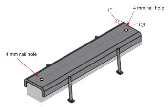
Figure 10 - HAC-TU cut in shorter sections and nail holes added
