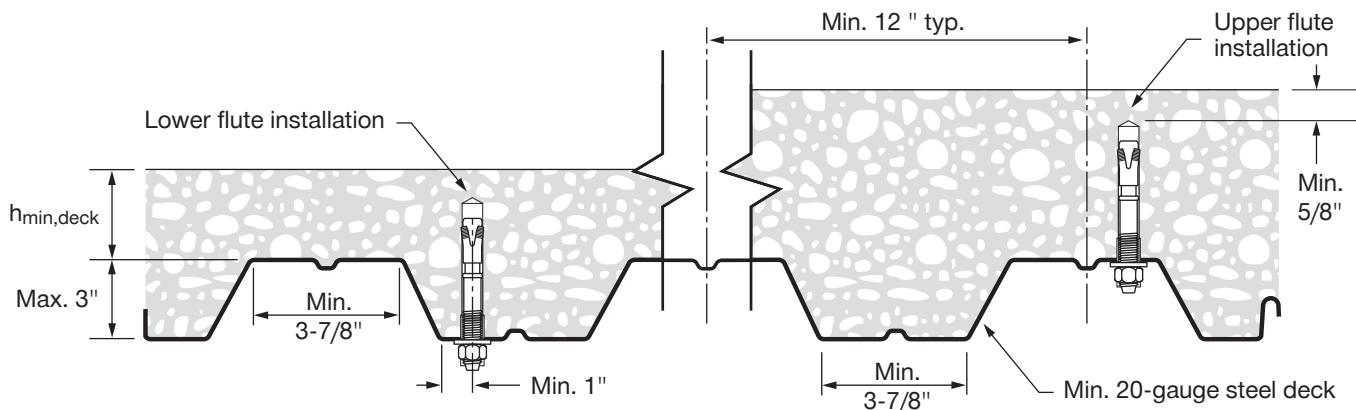
**Figure 4 — Installation in the soffit of concrete over metal deck floor and roof assemblies – B deck**
