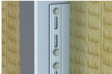
Fixed point: Screws positioned in the round holes
