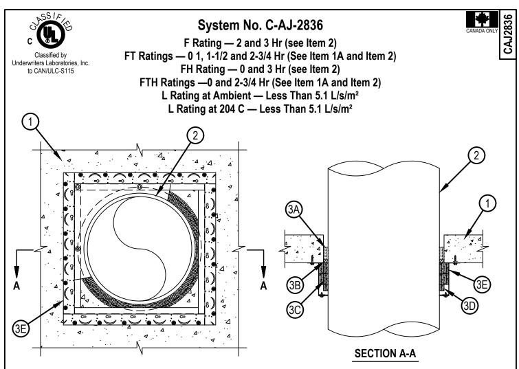
System tested with a pressure differential of 50 Pa or 2.5 Pa between the exposed and unexposed surfaces with the higher pressure on the exposed side (see table below).
