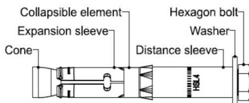
FIGURE 1—COMPONENTS OF THE HSL4 (BOLT VERSION SHOWN)
