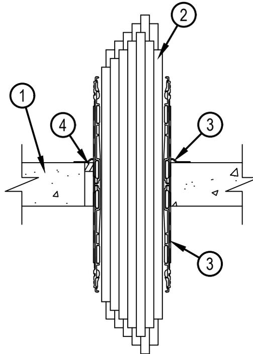
1. Floor or Wall Assembly — Min 2-1/2 in. (64 mm) thick reinforced lightweight or normal weight (100-150 pcf or 1600-2400 kg/m<sup>3</sup>) concrete. Wall may also be constructed of any UL Classified Concrete Blocks\*. Opening in floor or wall to be max 3 in. (76 mm) diam for 2" device and max 5 in. (127 mm) diam for 4" device.
