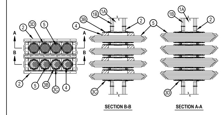
1. Wall Assembly — The 1 or 2 hr fire rated gypsum board/stud wall assembly shall be constructed of the materials and in the manner described within the individual U400, V400 or W400 Series Wall and Partition Designs in the UL Fire Resistance Directory and shall incorporate the following construction features:
