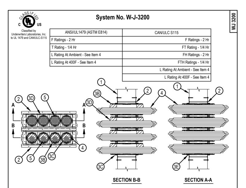
1. Wall Assembly — Min 6 in. (152 mm) thick reinforced lightweight or normal weight (100-150 pcf or 1600-2400 kg/m3) concrete. Wall may also be constructed of any UL Classified Concrete Blocks\*. Maximum opening sizes are specified in Table below. Opening may be oriented vertically or horizontally.
