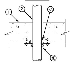
System tested with a pressure differential of 50 Pa between the exposed and the unexposed surfaces with the higher pressure on the exposed side.
