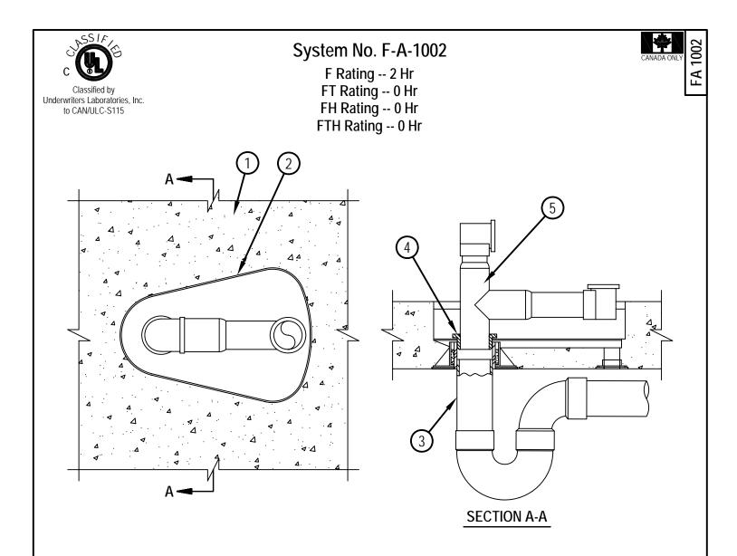
System tested with a pressure differential of 50 Pa between the exposed and the unexposed surfaces with the higher pressure on the exposed side. 1. Floor Assembly -- Min 114 mm (4-1/2 in.) thick reinforced lightweight or normal weight 1600-2400 kg/cu m (100-150 pcf) concrete.
