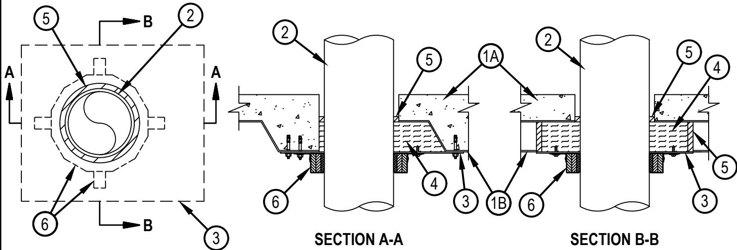
System tested with a pressure differential of 50 Pa between the exposed and the unexposed surfaces with the higher pressure on the exposed side.
