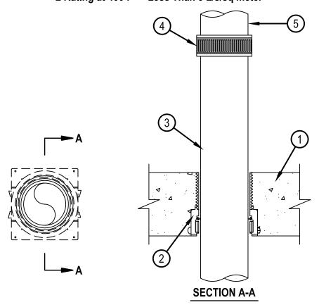
System tested with a pressure differential of 50 Pa between the exposed and the unexposed surfaces with the higher pressure on the exposed side. 1. Floor Assembly — Min 152 mm (6 in.) thick reinforced lightweight or normal weight (1600-2400 kg/m3 or 100-150 pcf) concrete.
