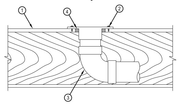
System tested with a pressure differential of 50 Pa between the exposed and the unexposed surfaces with the higher pressure on the exposed side.
