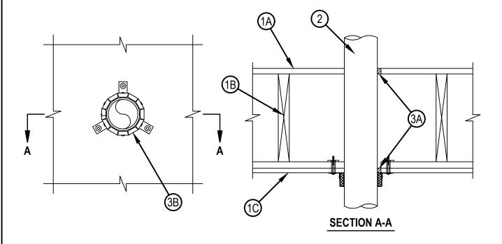
System tested with a pressure differential of 50 Pa between the exposed and the unexposed surfaces with the higher pressure on the exposed side.
