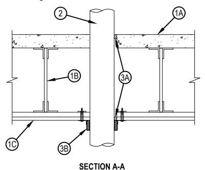
System tested with a pressure differential of 50 Pa between the exposed and the unexposed surfaces with the higher pressure on the exposed side.
