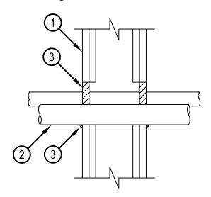
System tested with a pressure differential of 2.5 Pa between the exposed and the unexposed surfaces with the higher pressure on the exposed side.
