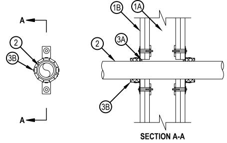
System tested with a pressure differential of 50 Pa between the exposed and the unexposed surfaces with the higher pressure on the exposed side.
