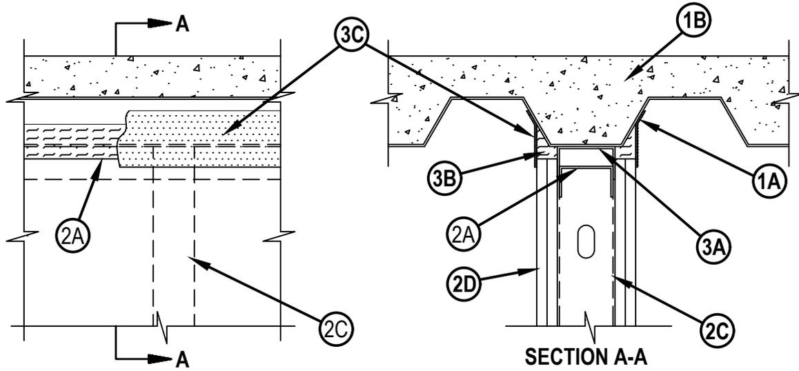
1. Floor Assembly — The fire-rated fluted steel deck/concrete floor assembly shall be constructed of the materials and in the manner described in the individual Floor-Ceiling Design in the UL Fire Resistance Directory and shall include the following construction features:
