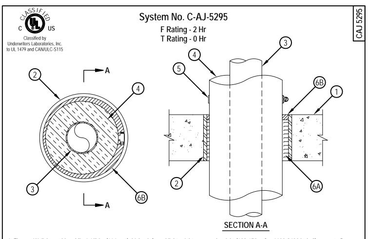
1. Floor or Wall Assembly -- Min 4-1/2 in. (114 mm) thick reinforced lightweight or normal weight (100-150 pcf or 1600-2400 kg/m3) concrete floor or min 5 in. (127 mm) thick lightweight or normal weight concrete wall. Wall may also be constructed of any UL Classified Concrete Blocks\*. Max diam of opening is 8 in. (203 mm).
