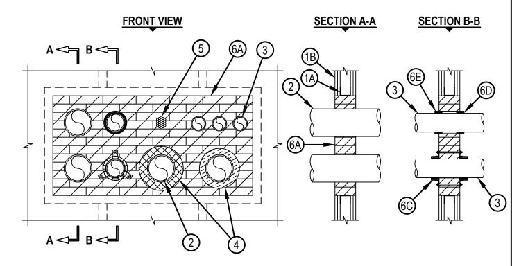
System tested with a pressure differential of 2.5 Pa between the exposed and the unexposed surfaces with the higher pressure on the exposed side.
