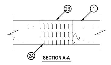
1. Floor or Wall Assembly — Min 4-1/2 in. (114 mm) thick reinforced lightweight or normal weight (100-150 pcf or 1600-2400 kg/m³) concrete floor or min 5 in. (127 mm) thick reinforced lightweight or normal weight concrete wall. Wall may also be constructed of any UL Classified Concrete Blocks\*. Floor may also be constructed of min 6 in. (152 mm) thick UL Classified hollow-core Precast Concrete Units\*. Max diam of opening is 6 in. (152 mm).
