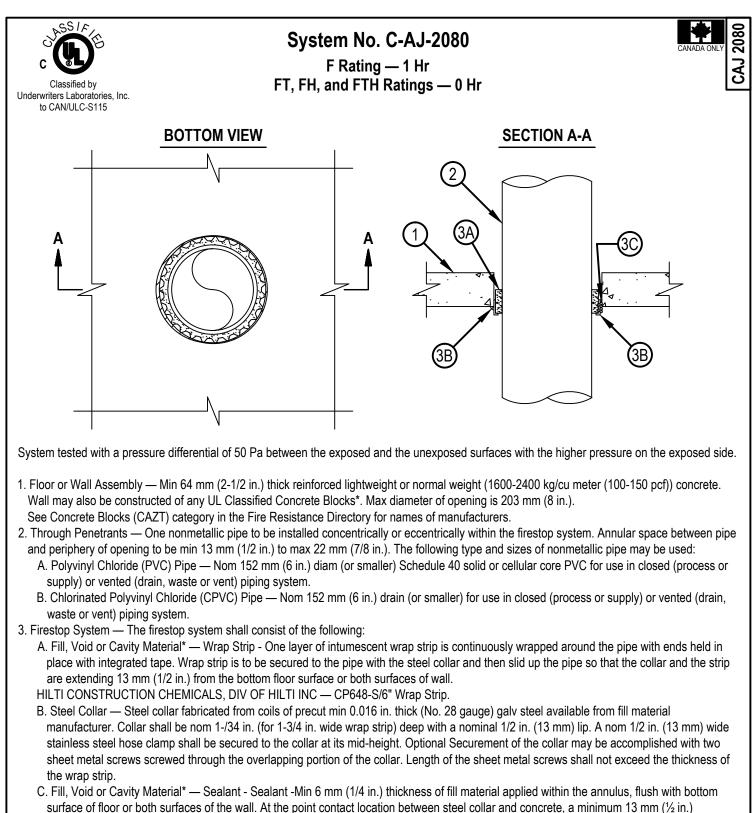
diameter bead of fill material shall be applied at the concrete/steel collar interface on the bottom surface of floor or on both surfaces of wall. HILTI CONSTRUCTION CHEMICALS, DIV OF HILTI INC — FS-ONE Sealant or FS-ONE MAX Intumescent Sealant
