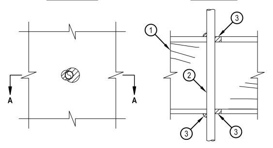
System tested with a pressure differential of 50 Pa between the exposed and the unexposed surfaces with the higher pressure on the exposed side.
