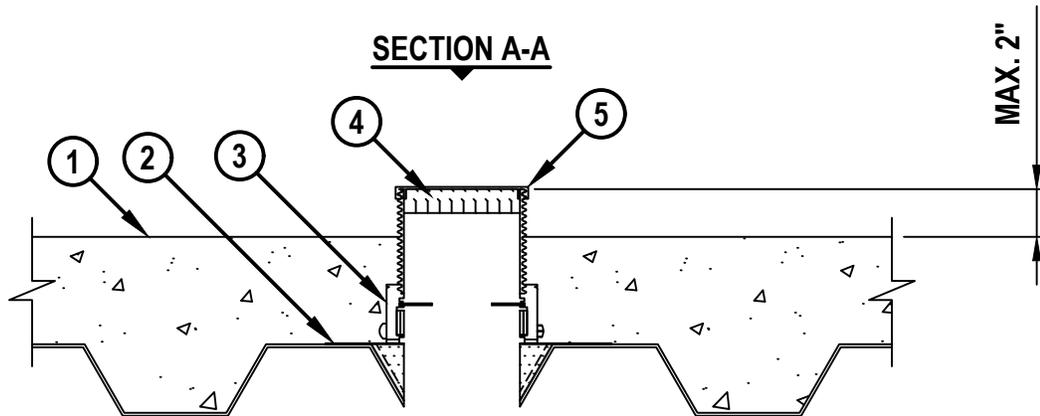
1. LIGHTWEIGHT OR NORMAL WEIGHT CONCRETE FLOOR ASSEMBLY (MINIMUM 4-1/2" THICK) OVER METAL DECKING (UL/cUL CLASSIFIED D900 SERIES) WITH 2" OR 3" FLUTED DECKS (3-HR. FIRE-RATING).
