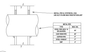
METAL PIPE THROUGH GYPSUM WALL ASSEMBLY (1-HR.) NOT TO SCALE E.4.1
