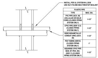
MULTIPLE PLASTIC PIPES THROUGH GYPSUM WALL ASSEMBLY 3 \(1-HR.) E.4.1 NOT TO SCALE
