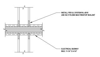
ELECTRICAL BUSWAY THROUGH GYPSUM WALL ASSEMBLY \(1-HR.) NOT TO SCALE
