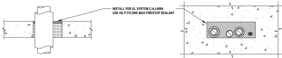
7 M.1.3 MULTIPLE PENETRATIONS THROUGH CONCRETE FLOOR (3-HR.) NOT TO SCALE
