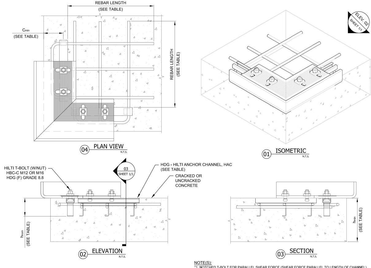
\*1. NOTCHED T-BOLT FOR PARALLEL SHEAR FORCE (SHEAR FORCE PARALLEL TO LENGTH OF CHANNEL) APPLICATIONS.
