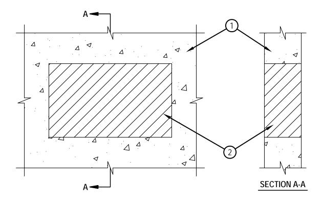
1. Wall Assembly — Min 4-3/4 in. and 6 in. thick reinforced lightweight or normal weight (100-150pcf) concrete for 1 and 2 hr fire rated walls, respectively. Wall may also be constructed of any solid or filled UL Classified Concrete Blocks\* Max area of opening is 450 in.2 with max dimension of 30 in.
