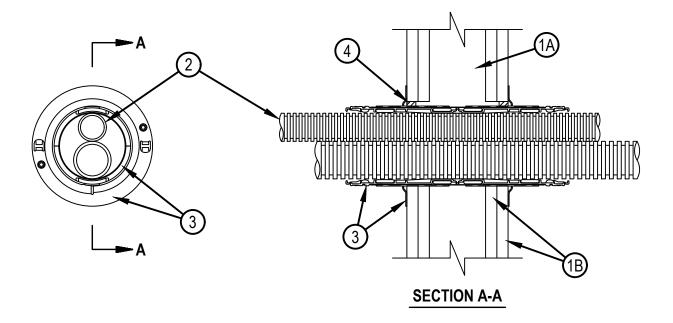
System tested with a pressure differential of 2.5 Pa between the exposed and the unexposed surfaces with the higher pressure on the exposed side.
