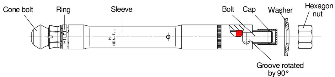
**Figure 2—Through-fastening anchor HDA-T and HDA-TR (Through-Setting)**
