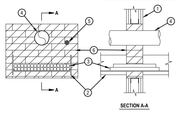
System tested with a pressure differential of 2.5 Pa between the exposed and the unexposed surfaces with the higher pressure on the exposed side.
