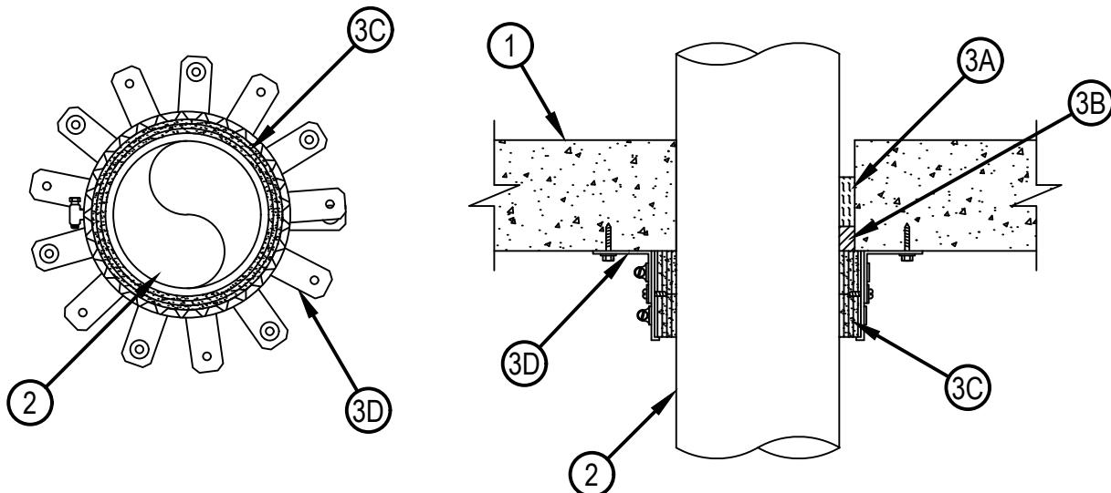
1. Floor or Wall Assembly — Min 4-1/2 in. (114 mm) thick reinforced lightweight or normal weight (100-150pcf) (1600-2400 kg/m<sup>3</sup>) concrete. Wall may also be constructed of any UL Classified Concrete Blocks\*. Max diameter of opening is 7 in. (178 mm).
