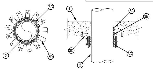
System tested with a pressure differential of 50 Pa between the exposed and unexposed surfaces with the higher pressure on the exposed side.
