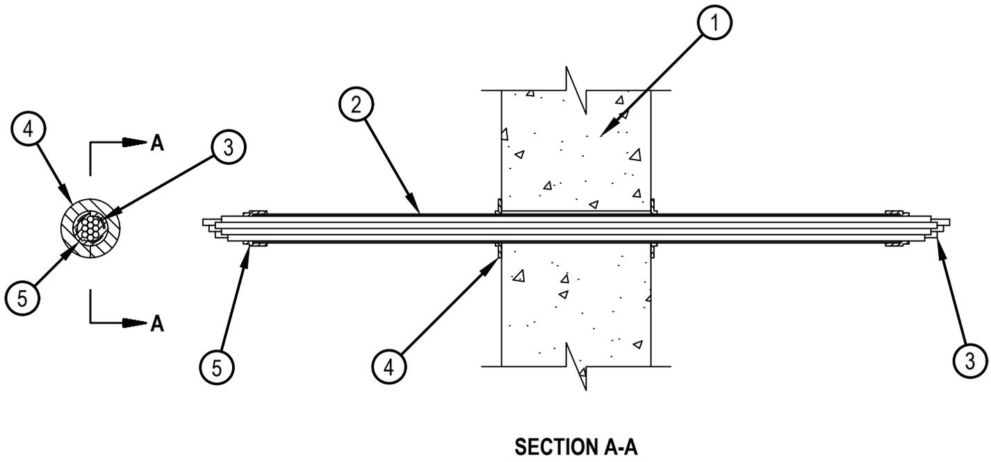
1. Wall Assembly — Min 6 in. (152 mm) thick reinforced lightweight or normal weight (100-150 pcf or 1600-2400 kg/m<sup>3</sup>) concrete Wall may also be constructed of any UL Classified Concrete Blocks\*. Max diam of opening is 1-1/8 in. (29 mm).
