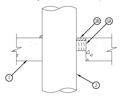
1. Floor or Wall Assembly — Min 4-1/2 in. thick reinforced lightweight or normal weight (100-150 pcf) concrete. Wall may also be constructed of any UL Classified Concrete Blocks\*. Max diameter of opening is 31-7/8 in.
