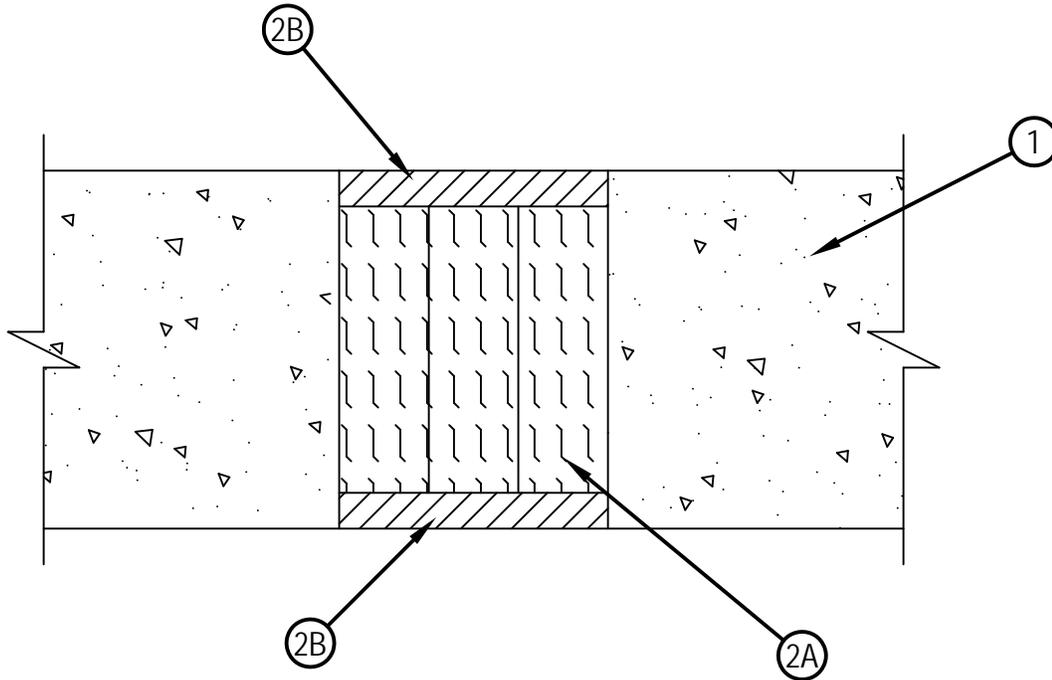
1. Wall Assembly — Min 4-1/2 in. (114 mm) thick reinforced lightweight or normal weight (100-150 pcf or 1600-2400 kg/m<sup>3</sup>) structural concrete. Wall may also be constructed of any UL Classified Concrete Blocks\*.
